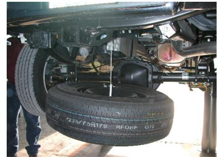
**STEP TWO** - MARKING AND CUTTING 4 INCH HOLE IN TRUCK BED FLOOR
