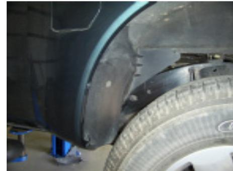
These locations are critical for the correct installation of this hitch, so measure, mark, and saw carefully. Make a 4" hole in this location using a 4" hole saw, or by marking a 4" circle and cutting it out with a saber saw equipped with a metal cutting blade.
