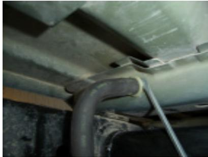
C) The inner fender guards toward the front of both rear fender wells will need to be removed to allow the installation of the hitch side plates. This is done by removing two screws and sliding the guard toward the tire. These guards will be replaced in step 10.
