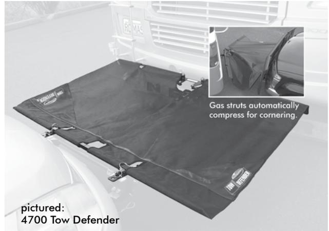
Gas struts automatically compress for cornering.
