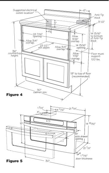
reach. Power cord access hole in cabinet should be a minimum  $1\,^{1/2}$ " diameter hole and deburred of all sharp edges.
