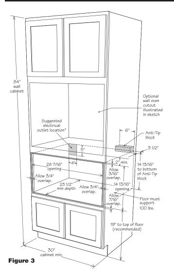
Figures 3,4 and 5 contain many Microwave Drawer measurements for reference when planning the drawer's location.
