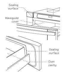
drawer, damaged drawer seals and sealing surfaces, broken or loose Microwave Drawer guides and dents inside the cavity or on the front side of the drawer. If there is any damage, do not operate the Microwave Drawer and contact your dealer or a SHARP AUTHORIZED SERVICER.
