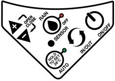
fan is turned on or off. On Manual Opening Models, pushing this key while in Auto Mode will exit Auto Mode, turn off the fan and the lid will stay in the position you selected. On Automatic Opening Models, this button will exit Auto mode, turn the fan off, and close the lid.
