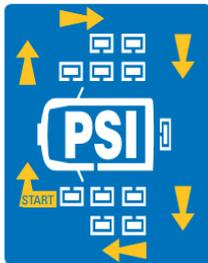
The front left tire will begin flashing. This is where the first sensor needs to be attached
