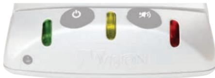
On the face of the monitor (Illustration C) you will find 3 different colored lights. These lights are designed to provide a quick reference to the status of your tires.
