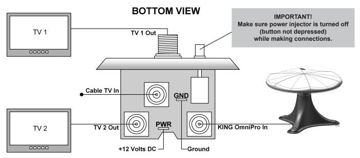
(+12 VDC and Ground require #10-12 female spade connectors)
