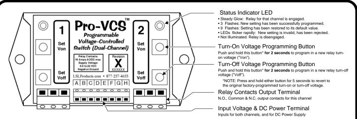
When DC power is first applied, the indicator LED(s)s will flash once to confirm that the unit is operating normally. At the same time, the contacts for the relay(s) are initially set in the normal (unactuated) position (i.e., the NC contact is closed).
