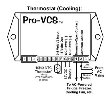
Thermistor This particular has а negative temperature coefficient (as denoted by the "NTC" designation) which resistance means that its decreases as it gets warmer. Thus, when connected as shown, it will produce a higher voltage in warmer temperatures (closing the NO relay contacts), or a lower voltage in cooler temperatures (closing the NC relay contacts instead).
