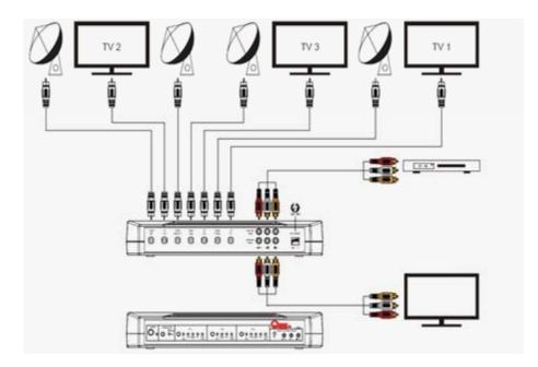
The QS53E model is equipped with a video modulator that allows you to hook up one composite video cable (Yellow, Red, White), to the back of the unit and play it through any of the attached TV locations on ch3 or ch4, depending on which LED is lit on the front of the unit in the section marked "MODULATOR". This allows you to hook up a DVD player, game system or any source with composite video (Yellow, Red, White) connections. Here is an example of use of the modulator with a DVD player.
