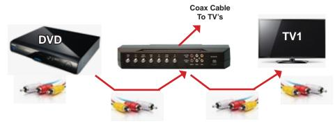
Take the composite video cable from the back of the DVD player and run to the "Video Input" on the back of the QS53E unit. Then run a composite video cable from the back of the QS53E unit from the "Video Output" to the "Video Input" on the back of the TV. Now you have created a loop that will take the video signal from the device hooked up to the QS53E "Video Input" and feed it to a receiver for audio or to the TV directly.
