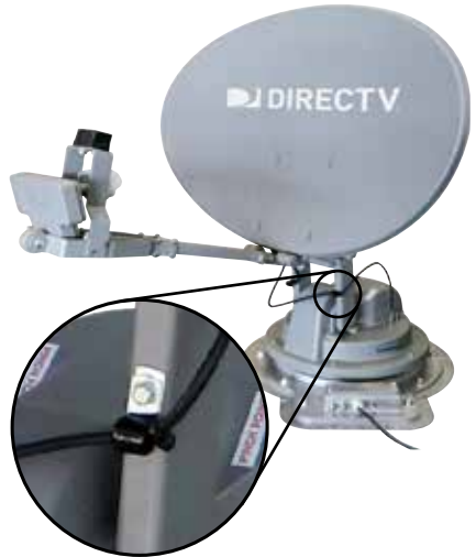
P-clamp installed 14" from ends of sheathed cables, next to zip tie on sheathed cables
