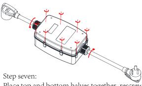
Place top and bottom halves together, rescrew all the screws, tighten down the cable gland connectors.
