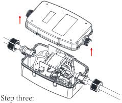
Carefully separate the top and bottom halves of the Power Watchdog Unit.
