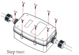
Unscrew the 8 Phillips screws (M3\*16) on the back side of the unit.
