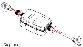
Loosen and unscrew the top and bottom cable gland connectors.
