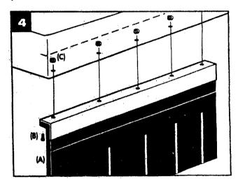
Fasten (A) Section to bumper using 5 of the (B) 1/4" Bolts as shown. Tighten nuts. Repeat for other (A) Section piece to finish installation.
