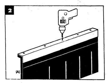
Mark five points on (A) Section with pen or pencil at which holes will be drilled. Drill five 1/4" holes in (A) Section at marked points. Repeat on other (A) Section.
