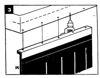
Align (A) Section under bumper to mark points at which to drill holes for mounting. Drill 1/4" holes at the five marked points on bumper. Repeat for other (A) Section piece.
