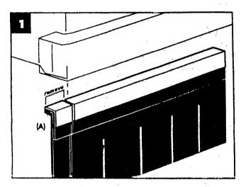
Measure length of bumper (NOTE: Take note of any extruding objects: hitch/muffler, that may interfere with (A) Section and trim accordingly). If necessary, trim off excess width from either edge of one of your (A) Sections with in snips or hack saw. File off burrs with a thin file Trim same amount from other (A) Section piece and file.
