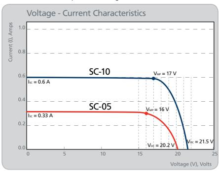
Fig. 1. Voltage versus Current characteristics.
