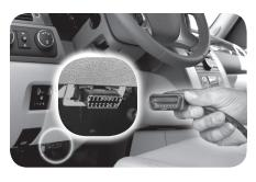
1. Plug the device into the OBDII port.
