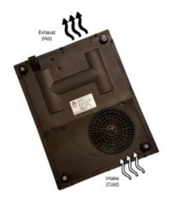
For proper air circulation, allow at least 3" of clearance from the bottom of the induction cooker to any shelving or storage. The underside of the countertop should not be closed off from the cabinetry underneath for better air flow.
