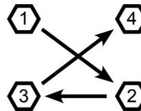
\*Always tighten and torque u-bolts in a cross pattern sequence.
