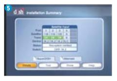
Verify that the check switch resulted in a switch type of DPP1K.2 and that there is a green 'OK' status on Satellite 110, 119, and 129.
