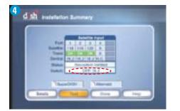
If the receiver shows a switch type of DPP1K.2, then a check switch test is not necessary. If it does not show a switch type of DPP1K.2, then make sure there are no checkmarks by "SuperDISH" or "Alternate," and select "Test."
