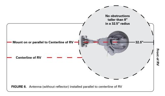
When installing the antenna on a rubber roof, Winegard recommends using Model SKA-004 roller plate, which is designed to create a solid landing area for the roller. If not using this plate, make sure that the roller does not come in contact with any rib supports or bubbles in the roof when in operation. Failure to do so may result in damage to the roof.
