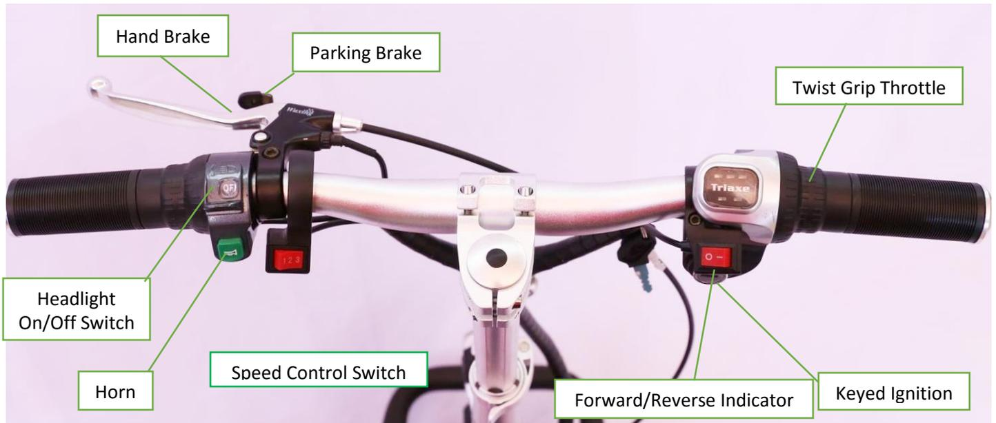
The Handlebar Control consists of a keyed ignition, twist grip throttle, forward-reverse indicator, horn, headlight on/off switch and handbrake that also acts as a parking brake.
