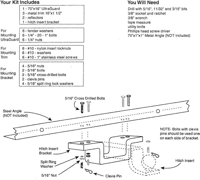
The hitch insert bracket shown can be used to mount the UltraGuard to any 2" hitch. The bracket slips under the hitch insert, (the insert has the ball mounted to it) and using a 70"x1"x1" steel angle (not included), the unit can be mounted to the hitch insert for easy removal and installation.
