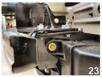
23. Place the backing plate on the bottom side of the frame webbing to align with drilled holes, insert the 3/8-16 x 1 1/2" hex bolts and 3/8" flat washers into this hole, tighten the 3/8-16 hex nuts and 3/8" lock washers. Reinstall the air baffle to its original position.
