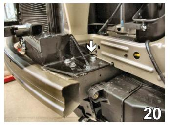
20. Slide bumper between frame and baseplate to align with existing mount locations. Insert two 8MM-1.25 x 30MM hex bolts with 5/16" lock washers and 5/16" flat washers and tighten. Tighten the bolt near the back of the baseplate, as indicated by the white arrow in the photo above. Do this to both sides of the vehicle.
