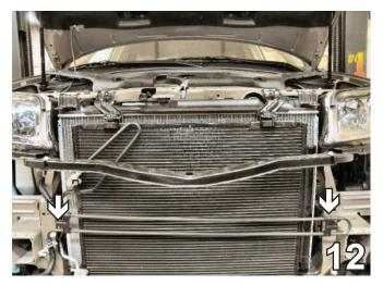
12. On the lower section of the radiator support, use a 10MM socket to remove the metric bolt of the coolant tubing bracket. Do this to both sides of the vehicle. Swivel the coolant line out of the way to clear the area for baseplate installation.
