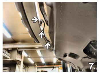
7. Behind the bumper, remove the temperature sensor from its clip. Also remove two pushpin connectors for the coax cable that are secured behind the bumper. Set temperature sensor and coax cable out of the way to be reinstalled later.
