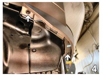
4. Just forward of the front tire, on the outermost bottom edge of fascia, remove two metric bolts using a 10MM socket, as indicated by the white arrow in the photo above. Do this to both sides of the vehicle. Set bolts aside to reinstall later.
