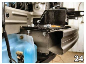
24. Place the backing plate on the bottom side of the frame webbing to align with drilled holes, insert the 3/8-16 x 1 1/2" hex bolts and 3/8" flat washer into this hole, tighten the 3/8-16 hex nut and 3/8" lock washers.
