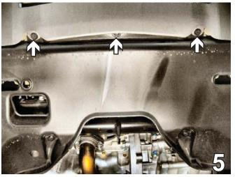
5. Remove three pushpins that run horizontally along the bottom of fascia, where the belly pan and fascia meet. Set bolts aside to be reinstalled later.
