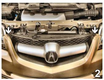
2. Between the headlight and the grille, on the top side of the fascia, remove two pushpins. Set pushpins aside.
