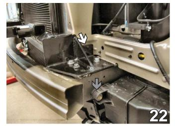
22. Align the nut plate with the drilled hole on the back side of the radiator support and tighten the 3/8-16 hex bolt and lock washer, as indicated by the white arrow in the photo. Do this to both sides of the vehicle. Using the 10MM socket, remove the metric bolt from the air baffle, as indicated by the grey arrow in the photo, and pull the air baffle down away from the frame.
