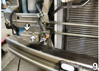
9. Using a 12MM socket, remove two metric bolts from the metal bumper bracket and one metric bolt underneath the metal bumper. Do this to both sides of the vehicle. Pull bumper forward to remove. Set metal bumper and bolts aside to reinstall later.
