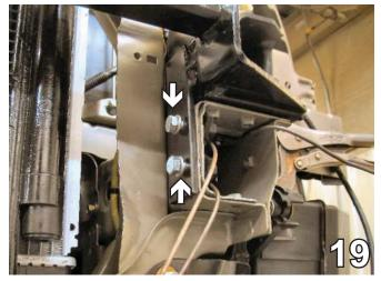
19. Insert the 3/8-16 hex bolts with the 3/8" lock washer through the baseplate holes on the side of the frame rail. Hand tighten bolts to the 3/8-16 nut plates placed on hex bolts through opening in frame end. Do this to both sides of the vehicle. Using diagonal cutters, cut all nut plate wires flush with the end of the frame. Be sure to apply LOCTITE Red to ALL bolts.
