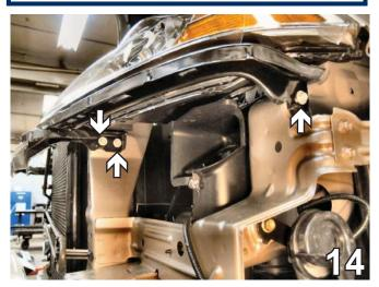
14. Using a 10MM socket, remove three metric bolts from the lower portion of the headlight assemblies bracket. One is located under the headlight, on the outermost edge of bracket. Two are located closer to the mid point of bracket that is secured to the radiator support. Do this to both sides of the vehicle.
