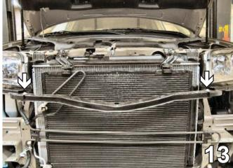
13. Using a 10MM socket, remove a metric bolt from either end of the headlight assemblies bracket. Set the bracket aside to be reinstalled later.
