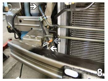
On the passenger's side remove one coax cable pushpin connector from the radiator support – just below the coolant tubing (see grey arrow). Release the clips from the coolant hose (see white arrows). Find one immediately behind the bumper, next to the frame rail. The other is found midway up the radiator support.
