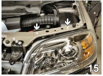
15. Using a 10MM socket. Pull the headlight assemblies forward to remove. Disconnect electrical connections. Set bolts and headlight assemblies aside to reinstall later.
