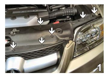
1. Remove 11 pushpins from the plastic above the radiator. Remove the plastic from the top of the radiator. Set pushpins aside to reinstall later.
