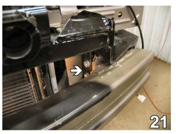
21. Tighten the bolts on the lower portion of the baseplate and all installed bolts in the top of the frame. Do this to both sides of the vehicle.
