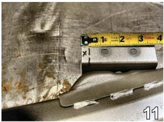
11. Mark and cut a section of the bumper bracket edge that faces toward the center of the bumper. Using the reciprocating saw, make a horizontal cut on the top of the bracket removing 3/8" from the end of the bracket. The cut travels the length of the top of bracket and down over the bracket lip about 1/4".
