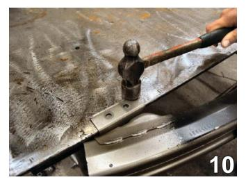
10. Lay the bracket of the metal bumper on a solid surface. Use a hammer to pound and flatten the rib on top of the bracket. Do this to both sides of the vehicle.
