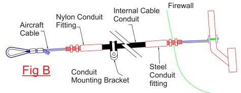
Step 2. Make sure there is no obstruction on the engine side of the firewall. Pull back the carpet and drill a 1/8" pilot hole allowing your drill bit to barely go through the firewall. If anything is interfering with this location drill another pilot hole. Remember to maintain as straight a line as possible.
