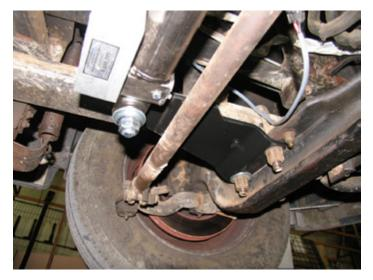
3. Slide the Anchor Bracket (Item 3) on the axle on the driver's side getting past the leaf spring. The plate offsets toward the center of the vehicle. Reinstall the existing washers and nuts and tighten to manufacturers specs.
