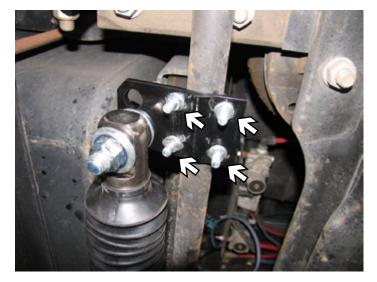
4. Install Tie Rod Bracket (Item 4) on the passenger's side tie rod using Items 8 or 9 (choose the appropriate U-Bolts for your application), according to drawing on page 3. DO NOT TIGHTEN. Item 4 may be rotated or flipped to insure Steering Control (Item 1) remains parallel to the ground.
