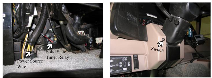
10. Install TruCenter Steering Control wiring according to instructions included in its package. Shown 1999 F-53 V-10 1.5 Tierod
