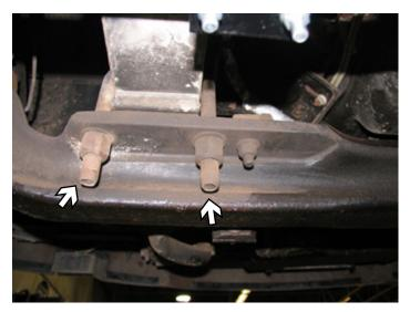
2. Using a 1 1/2" socket, remove two bolts and nuts from shock mount bar on the driver's side.
