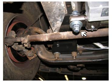
5. Install solenoid end of Item 1 to back of Anchor Bracket (Item 3) with 3 1/2" bolt, 3/4" flat washers and 1.59 flange nut (Items 5, 6 and 7), according to drawing on page 3.
