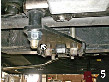
5. Install solenoid end of Item 1 to back of Anchor Bracket (Item 3) with 3/4"-10 x 5" bolt, 1-1/2" tube spacer, 3/4" flat washers and 3/4"-10 flange nut (Items 5, 6, 8 and 9), according to drawing on page #3. Tighten to 180-200 ft/lbs of torque. NOTE: Angled edge of Anchor Bracket should always be installed toward the outside of the chassis.
