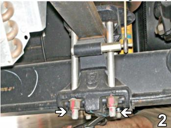
2. Using a 1-1/2" socket, remove two (2) bolts and nuts from shock mount bar on the driver's side.
