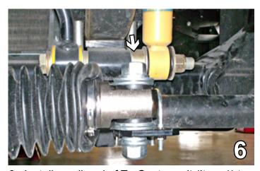
6. Install small end of TruCenter unit (Item 1) to top of Tie Rod Bracket (Item 4) with 3/4"-10 x 3-1/2" bolt, 3/4" flat washers and 3/4"-10 flange nut (Items 7, 8 and 9), see drawing on page 3. Allow enough slack for the Tie Rod Bracket (Item 4) to rotate to for alignment to the tie rod. DO NOT FULLY TIGHTEN.
