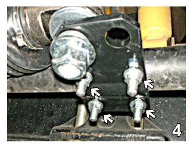
4. Install Tie Rod Bracket (Item 4) on the passenger's side tie rod using Items 10 or 11 (choose the appropriate U-Bolts for your application), according to drawing on page #3. DO NOT TIGHTEN. Item 4 may be rotated or flipped to insure Steering Control (Item 1) remains parallel to the ground.
