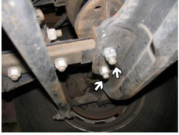
2. Using 1-1/8" socket, remove two (2) existing bolts and nuts from shock mount bar on the driver's side.
