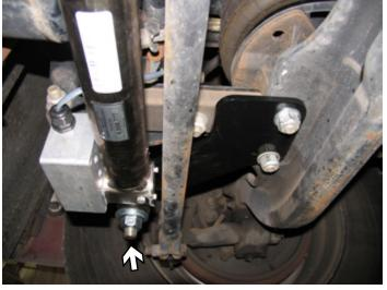
4. Install solenoid end of TruCenter to back of anchor bracket with a 3/4"-10 x 5" hex bolt, 1-1/2" spacer, 3/4" flat washers on the top and the bottom and 3/4"-10, 1.59 flange nut, torque to 180 ft/lbs.
