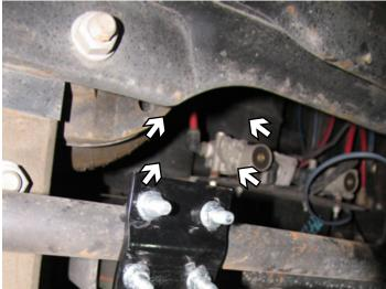
5. On the passenger's side, install the tie rod bracket using the appropriate U-Bolts for your application. DO NOT TIGHTEN. The tie rod bracket may be rotated to insure steering control remains parallel to the ground.
