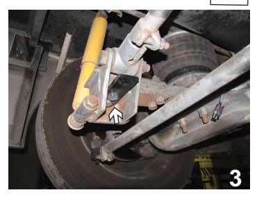
3. Slide the Anchor Bracket (Item 3) on the axle on the driver's side. Install the 5/8-11 x 3" bolts and 5/8-11 lock nuts and tighten to manufacturers specs.
