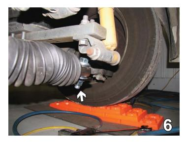
6. Install small end of TruCenter unit (Item 1) to the Tie Rod Bracket (Item 4) with 3/4-10 x 3 1/2" bolt, 3/4" flat washers and 3/4-10 flange nut (Items 7, 8 and 9), see drawing on page 3. Allow enough slack for the Tie Rod Bracket (Item 4) to rotate for alignment to the tie rod. DO NOT FULLY TIGHTEN.
