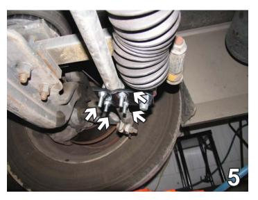
5. Install Tie Rod Bracket (Item 4) on the passenger's side using 3/8-16 x 1.375 U-bolts and 3/8-16 nuts, according to drawing on page 3. Tip the bracket down to avoid hitting other parts. DO NOT TIGHTEN. *Item 4 may be rotated or flipped to insure Steering Control (Item 1) remains parallel to the ground.*
