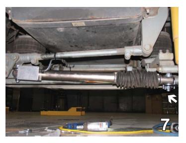
7. Tighten U-bolts (Item 10 or 11) on the Tie Rod Bracket (Item 4) to 25-35 ft/lbs of torque, while maintaining an even amount of threads extending past each nut.
