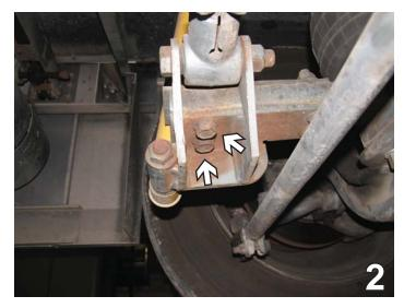
2. Underneath the vehicle using an 11/16" socket and wrench, remove two bolts and nuts from shock mount bar on the driver's side.
