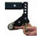
To stow, use hand to support hitch, rotate ball to storage position, then pull pin on hitch and rotate underneath.
