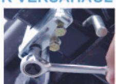
To attach the assembled VersaHaul to your class III or IV 2" receiver, first place the Anti-Tilt Lock Bracket as shown on the Main Tube. Be sure the flat side of the Bracket is facing the carrier. Insert the unit into your receiver. Insert hitch pin and on opposite side insert hair pin. Push the Lock Bracket all the way against the receiver then tighten all three \%" x 1\%" hex head screws with the \%6" Socket.
