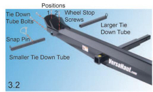
Insert the  $1\frac{1}{2}$ " x 19" Tie Down Tube through the Main Rail. Then, insert the  $1\frac{1}{4}$ " x 17" Tie Down Tube into the  $1\frac{1}{2}$ " x 19" Tie Down Tube. Lock into place with a Snap Pin. Secure the Tie DownTubes with two  $\frac{1}{4}$ " x  $\frac{3}{4}$ " Bolts. Do this for both ends (Figure 3.1 and 3.2).
