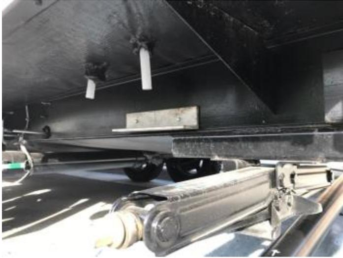
Here is the 2" aluminum angle attached to the frame on the driver side of the trailer. It was mirrored on the passenger side. This is what the 3" vent hangers are attached to. Then the 3" hangers fit really tight around the 4" landscape pipe. The thing is not going anywhere.
