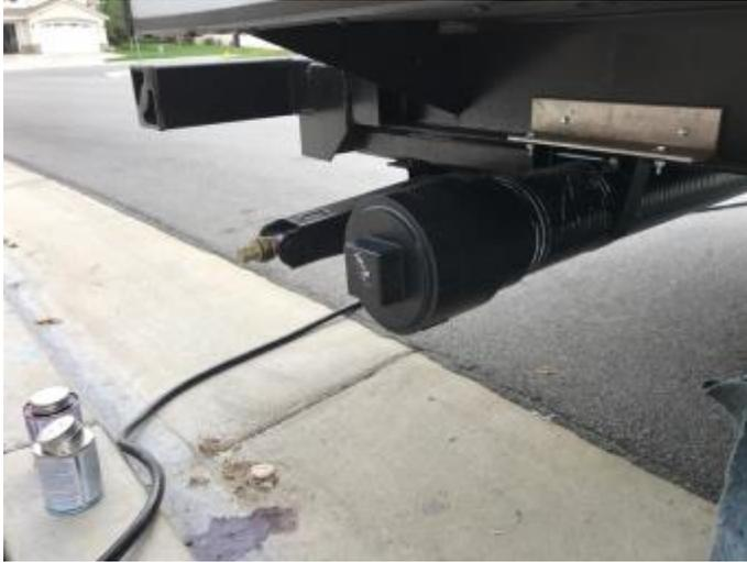
Here is the passenger side fit with the ABS cleanout. I had to adapt this with the 4" union for the drain pipe. This is styrene so I used ABS glue even though its white in appearance it worked fine. I like having the cleanout just in case the hose ever got stuck or I want to hose it out.
