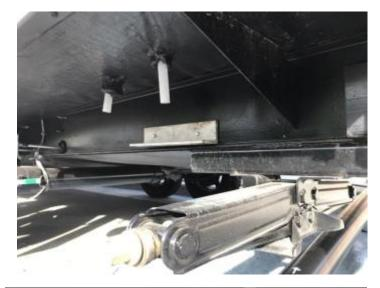
Here is the 2" aluminum angle attached to the frame on the driver side of the trailer. It was mirrored on the passenger side. This is what the 3" vent hangers are attached to. Then the 3" hangars fit really tight around the 4" landscape pipe. The thing is not going anywhere.
