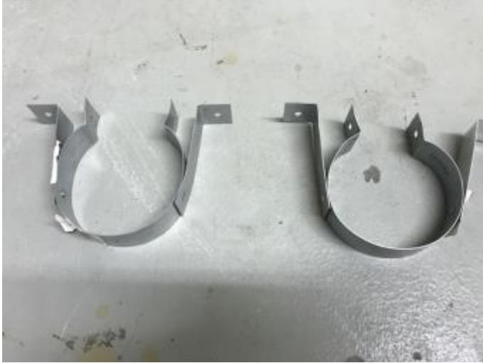
3" vent pipe hangers that are used to support the pipe under the trailer. The ORV is completely sealed underneath with a skin so all I had to support from was the outside frame.
