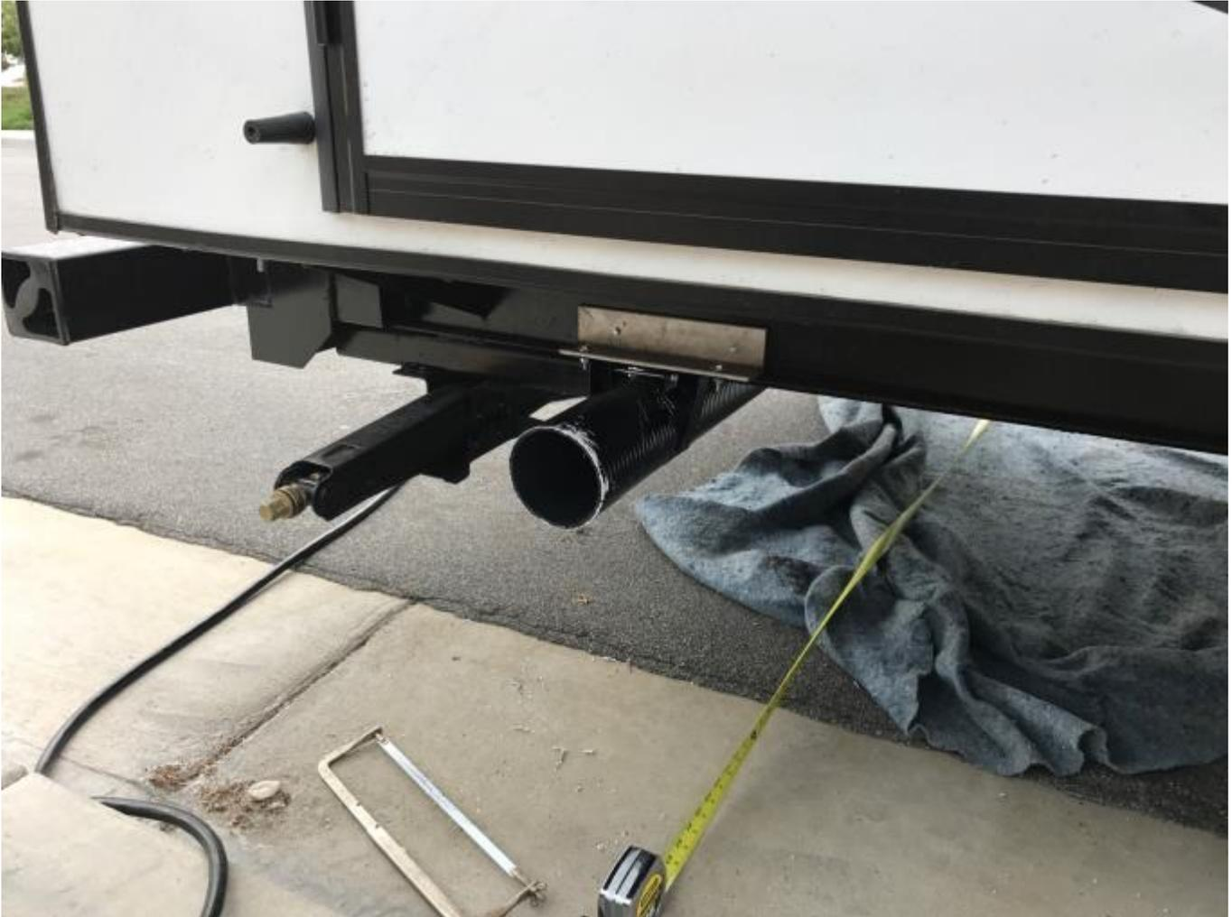
Here is the passenger side pipe after its mounted and cut. I needed 94" from the box to the end. This 94" was total and included the ABS cleanout I installed which is on the next page.
