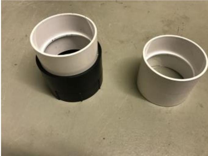
Here is the 4" landscape union and the 4" ABS cleanout fitting. The union fits directly inside the cleanout very tightly. So tightly I couldn't remove it to glue it. I hit a few times with a mallet and its never coming out. The 4" landscape pipe does not fit in the ABS fitting. I wanted this cleanout to access both sides of the storage pipe. I originally was going to cap it but opted for this.
