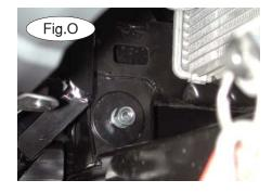
outside of the frame, bolt through the existing hole with a  $\frac{1}{2}$ " x 4" bolt (Fig.M). From the inside of the frame, thread a  $\frac{1}{2}$ " plate washer, lock washer and nut onto the bolt to secure it (Fig.O). Repeat for the other side.
