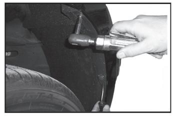
2. Remove one screw and two plastic push fasteners from each wheel well.
