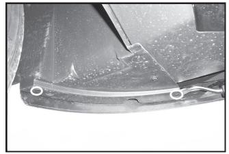
**3.** Remove four plastic push fasteners from bottom of fascia.
