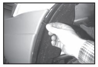
1. Insert plastic rivet into existing holes.
