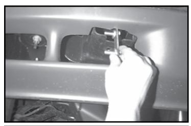
2. Insert bolt strip with two 3/8" flatwashers over each bolt, into frame, and through factory holes in outside of frame. Do this on each side.
