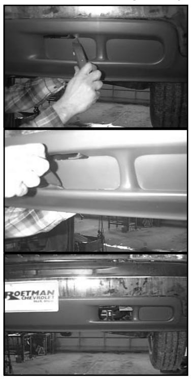
1. With a utility knife carefully cut out the two inside lower valance panels for the chevy pick-up as shown. For the GMC pick-up there is only one panel on each side, cut these panels out.
