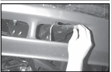
**4.** Insert the four threaded plates (two on each side). One is inserted through end of frame. The other is inserted through large hole and centered over it.
