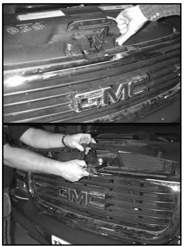
**2.** Open hood and remove four plastic push rivets on top side of grill. Lift plastic panel up and remove one bolt in right center of grill.
