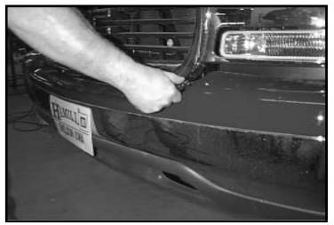
**4.** Turn two more 1/4 turn fasteners on bottom outer edges.
