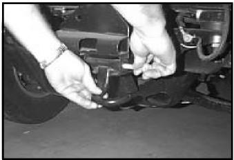
**8.** Remove tow hooks if equipped from each side. One bolt from bottom side of frame, and one cross bolt. Tow hooks and bolts will not be reused.
