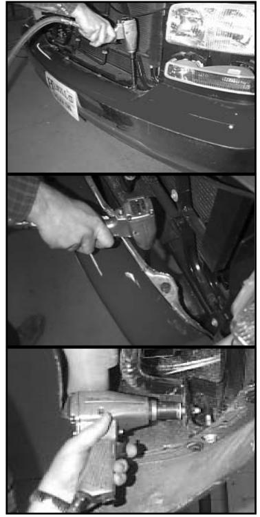
**6.** Through grill opening remove two top bumper bolts, and two bottom bumper bolts. Remove one bolt on each side that hold brace to bumper.
