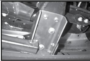
8. Plug mount (item #16) may be installed if desired in convenience holes on either chain anchor or as desired. **NOTE:** Excess material may be trimmed from bracket.
