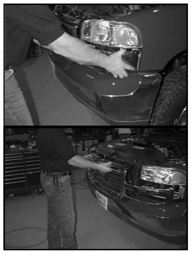
**5.** Carefully pull grill straight out, starting at turn signal area on each side.
