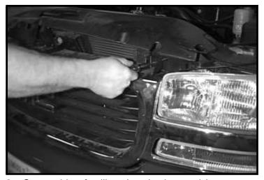
**3.** On outside of grill under plastic panel loosen two plastic 1/4 turn fasteners.
