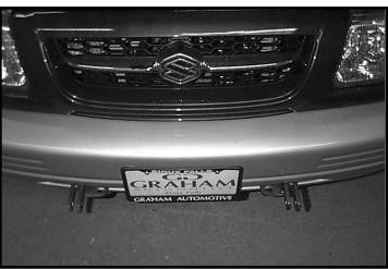
**10.** Install crossmember with 1/2" x 1-1/2" bolts, 1/2" lockwashers, and 1/2" hex nuts. (shims are included for crossmember if needed)
