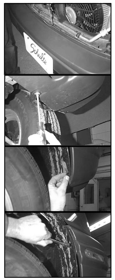
3. Remove bumper cover by removing plastic push fasteners from top side, three bolts from bottom side. Remove one plastic push fastener from inner fender to bumper cover, and one bolt from inner fender to bottom of front fender, on each side.
