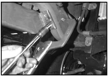
9. Install self-threading bolts at this time, and tighten all previously mentioned hardware to proper torque specifications. Remove C-clamps We require that "LOCTITE" Blue" be used on all bolts.
