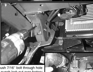
7. Install right and left frame mounts. Put proper side up and push 7/16" bolt through hole and start 7/16" lockwasher, and hex nut. Start 10mm x 1.25 punch lock nut over factory stud. Push mount up so angle is flat on front of frame, and clamp with C-clamp. Snug previously mentioned fasteners. Drill 5/16" holes through frame using mount as a template (three on each mount).
