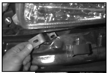
8. Remove top bumper bolt on each side and install brace with 8mm x 1.25 x 25mm bolt, 8mm lockwasher, and 8mm fender washer. Secure bottom of brace to frame mount using 3/8" x 1-1/4" bolt, 3/8" lockwasher, 3/8" flatwasher, and 3/8" hex nut. We require that "L@CTITE" Blue" be used on all bolts.
