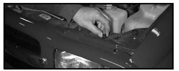
Remove grill by opening hood and removing plastic push fasteners from top of grill.
