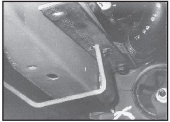
10. Remove front motor mount bolt on left side. NOTE: Remove only ONE motor mount bolt at a time. Install left stabilizer bracket using a 10mm x 35mm hex bolt and flatwasher in place of the factory bolt. Place a 1/2" x 1-1/4" hex head bolt and flatwasher down from top through opposite end of bracket and secure with 1/2" hex nut and lockwasher.
