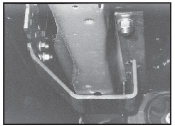
11. Secure front of bracket to Left Pod using two 3/8" x1-1/4" hex head bolts from front side and a 3/8" hex nut with lockwasher. Tighten the two bolts previously installed in rear of bracket then tighten front bolts. Always use " LOCTITE Blue" on threads.
