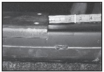
8. Position inside edge of Pod 2-5/8" from inside edge of bumper slot. Clamp pods in place and drill eight 3/8" holes in bumper. Secure pod using eight 3/8" x 1-1/4" hex head bolts, lockwashers and four inside nut strips. Always use " LOCTITE. Blue" on threads.
