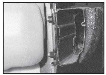
**6.** Mark bumper location on bracket before removal. Remove four nuts that attach the bumper using a 15mm wrench.
