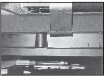
13. Install air dam snug with two outside bolts, mark air dam to cut lower bracket notches. Remove air dam, cut notches and replace air dam. Secure with six bolts that were removed earlier.
