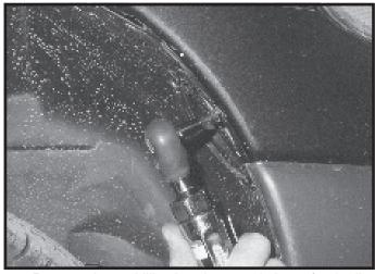
2. Remove three phillips head screws in inner fender lip, on both sides of the vehicle.
