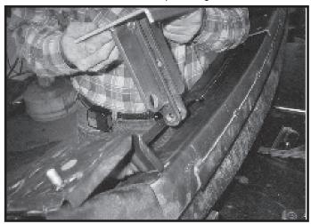
7. Insert Left and Right Base Plate Pods, so ears are pointed straight forward, into rear of front bumper as shown, lip of pod must be on top of bumper.
