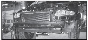
Carefully remove fascia panel from vehicle. Remove six bolts that secure air dam/inner support with 10mm socket and remove air dam.
