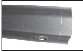
7. Vehicles that are equipped with tow hooks, cut one inch off end of facia.
