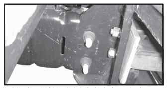
5. Put four 7/16" x 1-1/4" bolts in from the front and 7/16" Flatwasher, 7/16" lock washers and 7/16" nuts on back of bumper flange. NOTE: Check front page for correct right and left pull pod positions (chain anchor hole towards outside). Use LOCTITE® on all bolts. Adjust pods and tighten bolts according to bolt chart on front page.
