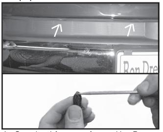
Open hood for ease of assembly. Remove bumper filler panel, by removing four plastic push fasteners from underneath front side of filler panel. If the phillips head plastic screw won't turn out, push plastic stem down from backside with small blade screwdriver, then pull out fastener.
