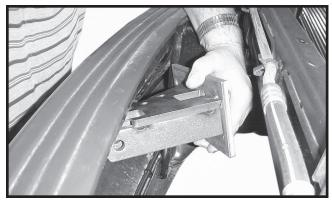
Install left and right pull pods by putting in from the back of bumper through filler panel/tow hook opening and slide over to mounting holes.
