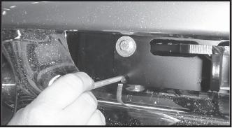
4. On some 1500's three holes may need to be drilled on each side. Bolt pods on with outside top bolts, mark other three holes and drill.
