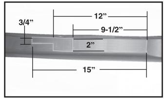
6. Mark panel by measuring 9-1/2" and 12" from edge of center panel hump and making two 2" vertical line from inner top panel edge. Then measure from hump 15" and mark a 3/4" vertical line down from top panel edge. You should have an outline marked on both sides of hump as shown in picture. Carefully cut out panel so pull ears may pass through and reinstall panel.
