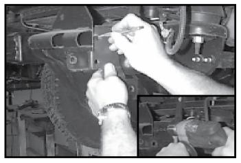
**2b.** If vehicle does not have two vertical holes on outside of frame, these will have to be drilled now. Hold side support brace up to side of frame aligning bottom holes. Mark through slotted hole onto frame. Center punch in center of marked slot and drill 7/16" hole. Bumper may have to be removed to drill the top hole, depending on equipment available.
