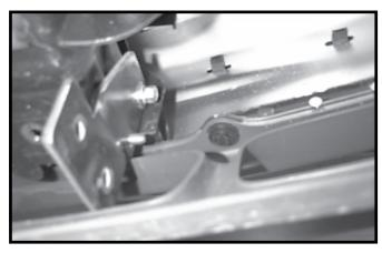
3. Attach right and left side support brackets with 3/8" flatwashers, 3/8" lockwashers, and 3/8" hex nuts. We require that "LOCTITE. Blue" be used on all bolts. Note: See diagram on front page for washer locations. Do not tighten nuts at this time.
