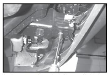
On some models a plastic filler panel behind tow hooks will need to be removed. Filler panel will not be reused. Remove tow hooks from each side. One bolt from bottom side of frame, and one cross bolt. These tow hooks and bolts will not be reused.
