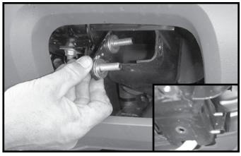
**2a.** Insert bolt strip with two 3/8" flatwashers over each bolt, into frame, and through factory holes in outside of frame. Do this on each side.
