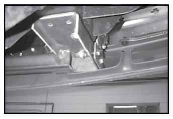
6. Attach side support brackets to baseplate with two 3/8" x 1-1/4" bolts, lockwashers, and hex nuts. We require that "L@@TITE. Blue"be used on all bolts. Tighten all bolts at this time.
