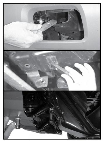
4. Insert the four threaded plates (two on each side). One is inserted through end of frame. The other is inserted through large hole and centered over it. On Avalanche, temporarily remove facia support brace by removing four bolts.
