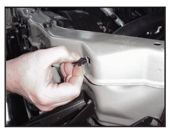
**3.** Release four plastic fasteners from vehicle and put back in grill for later installation.
