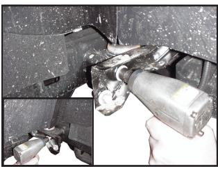
5. Remove two bolts from each side (unplug fog lights if equipped) and set bumper aside.
