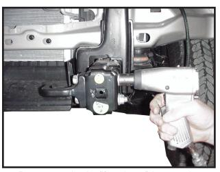
Remove tow hooks (if equipped) by removing two bolts on each side, bolts and tow hooks will not be reused (holes may need to be drilled for some models).
