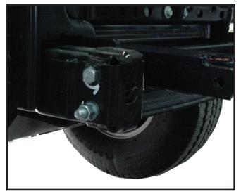
10. Use longer bolts (12mm-1.75 x 100mm Gr. 8.8) if no drilling is needed, slide baseplate between frame horns(If there is a gap between frame horns and baseplate insert shim as shown on front page), top bolt on each side will go inward and bottom bolt will go outward.
