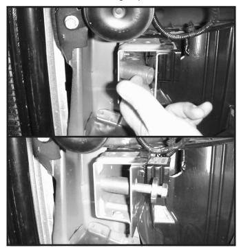
7. Install spacer bushing inside frame and hold in place with 1/2" x 3-1/2" bolt and heavy frame washer. NOTE: Don't stick 1/2" bolt all the way through so base plate can slide on.
