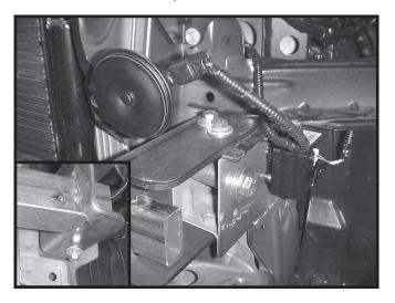
9. Install two 8mm-1.25 x 25mm bolts, 8mm lock washers and 8mm fender washers on top of each side and one 8mm-1.25 x 25mm bolt, 8mm lock washer and 8mm fender washer on bottom of each side. Do not tighten bolts yet. Put 1/2" bolt all the way through other side of base plate and install 1/2" lock washer and 1/2" hex nut. Tighten 1/2" bolts first then tighten 8mm bolts.
