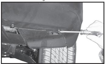
2. Remove six plastic push fasteners from underneath facia front.
