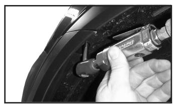
3. Remove two screws from each side, facia to fender, by going through wheel well.
