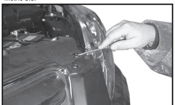
1. Open hood and remove six plastic push fasteners from across top of grill and facia.
