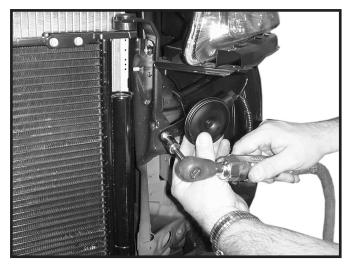
6. Relocate horn on each side, from straight down to outwards. Horn wiring clip will have to be removed from its hole so horn can be loosened and turned according to picture.
