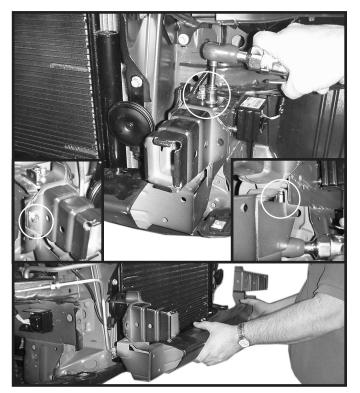
**5.** Remove facia support tin, four bolts on passenger's side and three bolts on driver's side. This assembly and bolts will not be reused. **NOTE:** Some models may have a temp sensor located on tin support, remove clip and relocate.
