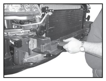
**8.** Slide base plate on frame horn until the top two bolt holes a lined up on each side.
