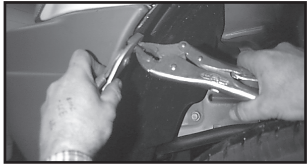
2. Use pliers as leverage tool for vise grip.
