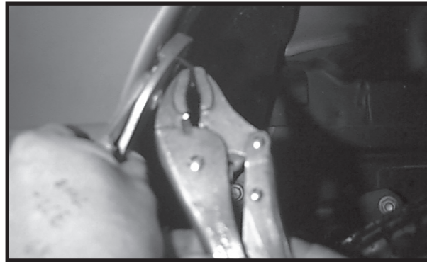
3. Use vise grip on rivet, and roll on pliers as shown.
