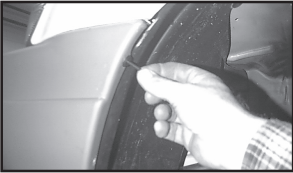
1. Insert plastic rivet into existing holes.
