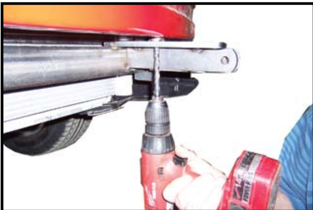
12. Drill two holes up through bumper. Insert supplied 3/8" bolts, lock washers, flat washers and nuts and tighten. Use blue LOCTITE on all bolts and tighten all bolts according to chart on front page.
