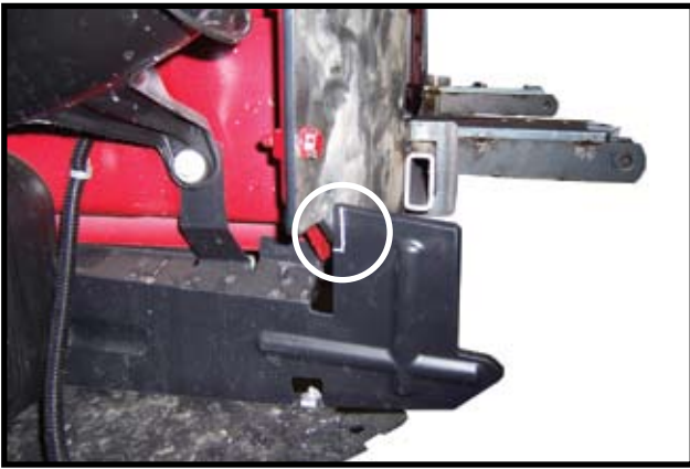
10. Notch plastic 1/4" on each side as shown above.
