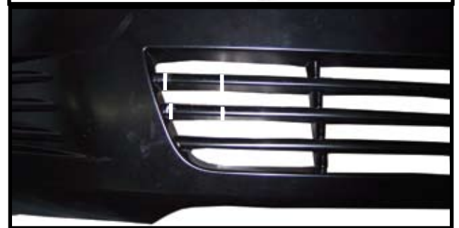
13. Notch grill and bumper tabs as shown above. NOTE: On some models with fog lights grill insert may be removed to cut.
