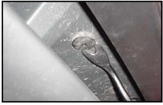
**4.** Remove four plastic push fasteners from middle of fascia, under bumper.
