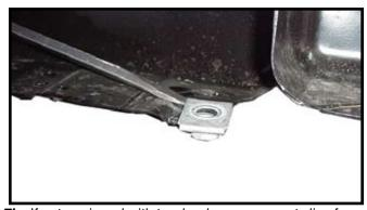
**7b.** If not equipped with tow hooks, remove nut clips from bumper. Nut clips will not be reused.
