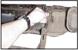
**8.** Remove plastic panel from inside of bumper. This will not be reused.
