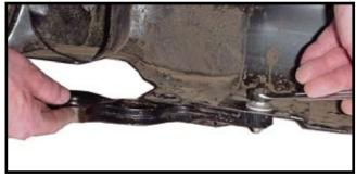
**7a.** After bumper is off, remove both tow hooks, if equipped, from bottom side of bumper. Tow hooks and tow hook bolts will not be reused.
