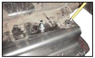
9. Bolt base plate to bottom side of bumper, using two 3/8" x 1-1/4" bolts, 3/8" lock washers and 3/8" nuts. Tighten these bolts when large hole in base plate is centered with large hole in bumper.
