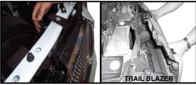
1a. Open hood, from behind release clips with needle nose pliers, carefully pull grill on top to release. On Trail Blazer also pull on bottom straight out to release, set grill aside and go to step 2.
