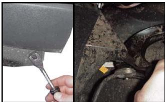
5. Remove one push fastener from each side at bottom of fascia, at end of air dam. Also, one push fastener from each side, inside of fascia to bumper. Unplug fog lights and clearance lights if equipped and carefully pull Envoy fascia straight off.
