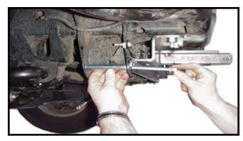
**11.** Put 1/4" spacer washer behind baseplate's slotted hole on each side and use 7/16" x 5-1/2" bolts, 1/4" spacer washers, 4" bushing spacers, 7/16" lock washers and 7/16" nuts. Tighten these bolts.
