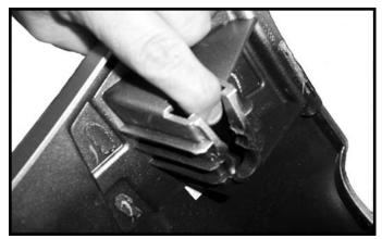
**5a.** On Trail Blazer models release clip on backside of fascia and pull straight off.
