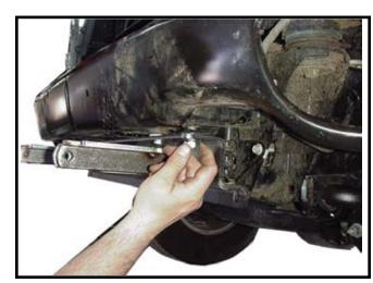
**10.** Put bumper back on and install both large bolts previously removed and tighten using the 14mm nuts provided. **NOTE:** Use **LOCTITE.** Blue on all bolts and tighten according to chart on front page.
