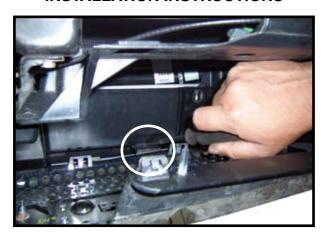
**1b.** On Envoy carefully release tab on bottom of grill while pulling up on grill. Rest grill on top of engine compartment if equipped with headlight washers.
