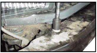
**6.** Remove bumper by removing large bolt from top side, one on each side.
