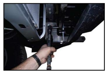
6. Insert center channel and bolt to each pod with supplied 3/8" x 1-1/4" hex head bolts, 3/8" lockwashers, and 3/8" hex nuts. *NOTE: Use Blue L@*€*TITE*<sub>●</sub> *on threads and tighten bolts according to bolt chart on front page.*
