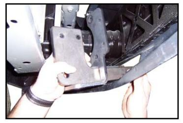
**3.** Pull facia down and insert pod on to bumper bolts on each side.
