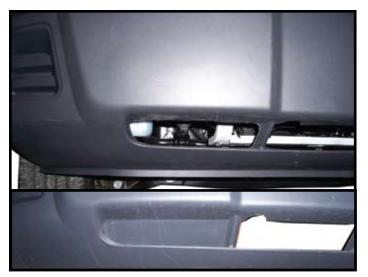
1b. Some models will need the outside portion of facia cut out for baseplate pull ears to pass through. See picture.NOTE: Tow hooks must be removed if equipped.
