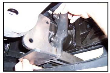
Put bumper nuts back on and tighten.
