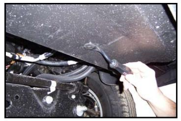
**1a.** Models equipped with radiator shroud, remove plastic push fasteners from the radiator shroud. Set shroud aside for later notching.
