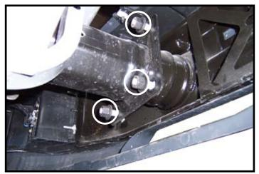
2. Remove three nuts from bumper brackets, two from the bottom one from the inside top.
