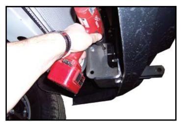
5. Drill 5/16" holes in frame and screw in bolts.
