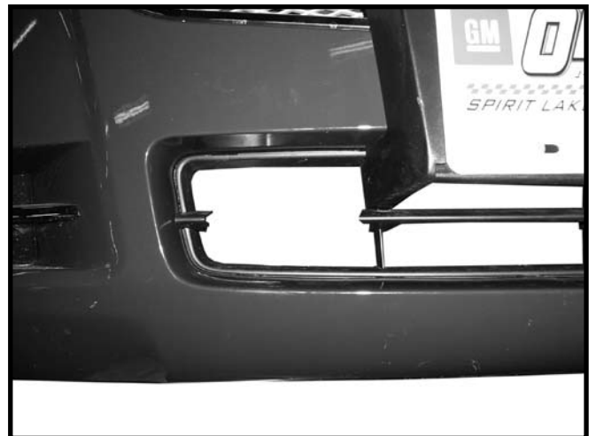
16. Notch plastic on front fascia for pull ears as shown above. Reinstall fascia, plastic filler panels and all hardware. Install horn with longer supplied metric bolt, washer, and lockwasher.
