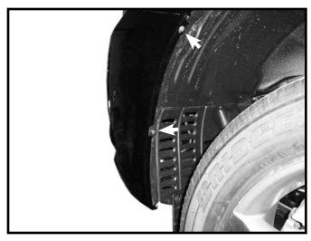
**4.** Remove one plastic push fastener and one screw from wheel well.
