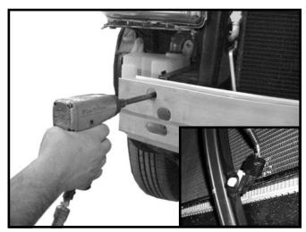
6. Remove styrofoam and bumper, three bolts on each side. These bolts will not be reused. If equipped with temp sensor, switch to back side of mount.
