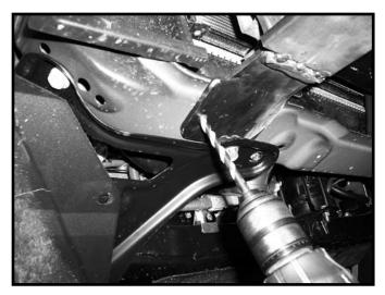
**9.** Drill 5/16" hole, using base plate as template, and fasten with 3/8" x 1" Thread cutting bolt. Do this on both sides.
