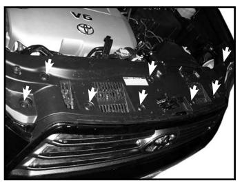
1. Open hood and remove eleven plastic push fasteners from top of facia filler panel above grill and set aside..
