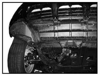
**3.** Remove plastic belly pan and all of its fasteners. Also remove fasteners from wheel well extension to front of facia.
