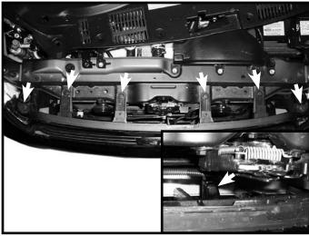
2. Remove two bolts and four plastic push fasteners top of grill, and one plastic push fastener from the bottom backside of grill. You can gain access from top of facia by hood latch.
