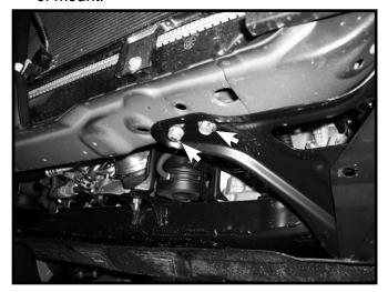
7. Remove one bolt and nut on each side from brace which is attached to bottom of radiator core support. (This bolt will not be reused). Slide base plate on with bottom under the brace. Start a 10mm-1.25 x 30mm bolt with 10mm washers (narrow washers).
