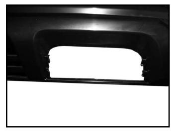
**10.** Cut out facia grill bars out on each side as shown in picture, for pull ears to pass through.
