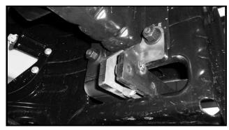
**6.** Place pull pod on the 3 bolts studs and replace 3 nuts leaving nuts loose Repeat steps 3, 4,5 and 6 for opposite side.
