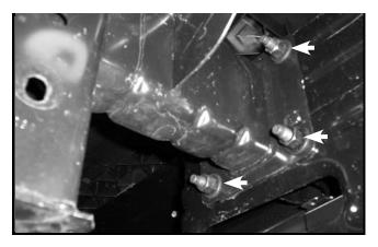
**3a.** If NOT equipped with tow hooks remove three nuts from back of bumper.
