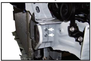
9. Place two 5/16 x 1 bolts thru holes. On inside of frame place two 5/16" flat washers, two 5/16" lock washers and two 5/16" nuts. Use blue **L@€717E**<sub>®</sub> on bolts and tighten all bolts according to chart on front page.
