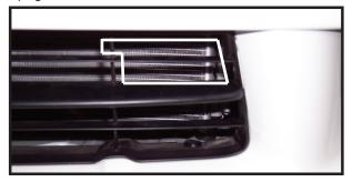
13. For sport model trim lower grill as shown for pull ears to pass thru. Minor adjustments may be needed for desired fit.
