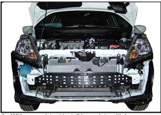
11. With an assistant install baseplate with bumper over top of baseplate onto vehicle re-using the eight bolts removed in step 6. Use blue LOCTITE<sub>®</sub> on all bolts and tighten all bolts according to chart on front page.
