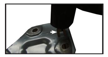
Flatten the hanger tab on back of the bumper with a hammer or remove with pliers or sander.
