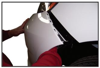
**5.** Pull on the outer corner of the facia outward and down to Remove Facia. Push from inner fender under headlights. Unplug fog lights if equipped.
