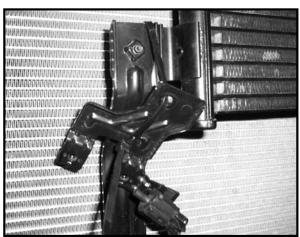
**6.** Remove the one bolt that holds the mount and temp sensor and attach it with the zip tie provided to the cooler mount above its location.;
