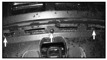
**2.** Remove three plastic push fasteners from the bottom of the facia.
