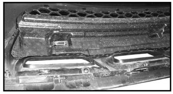
**12.** Due to vehicle differences the facia may not fit properly over the bumper if this happens remove the foam insert on the back of the facia.
