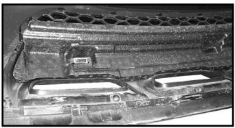
**18.** Due to vehicle differences the facia may not fit properly over the bumper if this happens remove the foam insert on the back of the facia.
