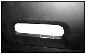
**17.** Test fit the facia. The bottom lip of the hole that the baseplate protrudes through may need to be trimmed slightly. Trim to desired fit and look.
