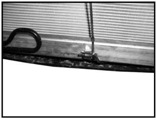
**14.** Use nylon tie to fasten temp. sensor to crossmember as shown in picture.
