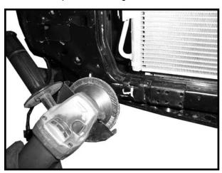
**8.** Grind off plastic from radiator bracket as marked in picture.
