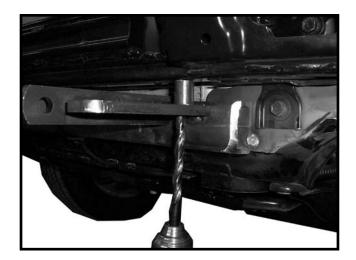
16. Using the baseplate as a template use a 13/32" drill bit to drill holes in the bottom of the bumper. Place the 3/8" x 2-1/2" bolt with two 3/8" flat washers, one 3/8" lock washer and one 3/8" nut on each side. The shim may be needed between bumper and tube. NOTE: Use blue LOCTITE on all bolts and tighten all bolts according to chart on front page.
