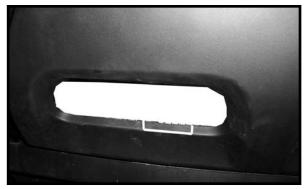
**11.** Test fit the facia. The bottom lip of the hole that the baseplate protrudes through may need to be trimmed slightly. Trim to desired fit and look.
