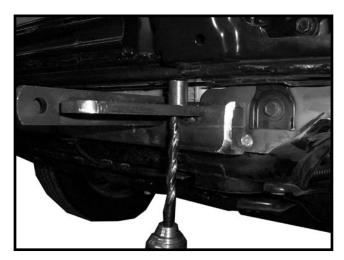
10. Using the baseplate as a template use a 13/32" drill bit to drill holes in the bottom of the bumper. Place the 3/8" x 2-1/2" bolt with two 3/8" flat washers, one 3/8" lock washer and one 3/8" nut on each side. The shim may be needed between bumper and tube. NOTE: Use blue LOCTITE on all bolts and tighten all bolts according to chart on front page.
