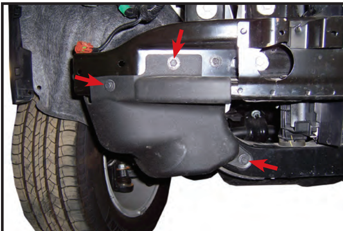
11. Remove three bolts and remove plastic bumper shield. Repeat for other side of bumper.
