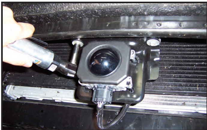
18. IF EQUIPPED WITH ADAPTIVE CRUISE CONTROL Remove two screws from adaptive cruise control sensor and let hang.
