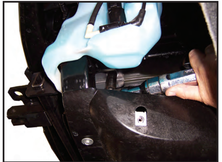
17. With an assistant, install baseplate up against bottom of frame. Fasten using four 10mm flat fender washers, 10mm lock washers and 10mm-1.50 x 35mm bolts, thread into existing threaded holes in frame, NOTE: Use blue LOCTITE® on all bolts and tighten all bolts according to chart on front page.
