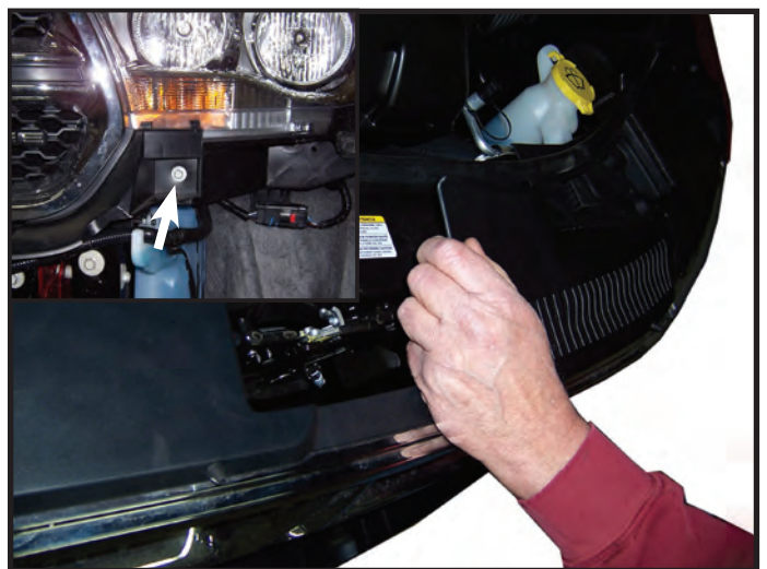
12. Remove grill assembly by pulling up on plastic on each side on top and remove one bolt on each side under headlight and set aside.
