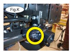
5. Place a  $\frac{1}{2}$ " lock washer over a  $\frac{1}{2}$ " x  $\frac{1}{4}$ " bolt. Place a  $\frac{3}{16}$ " x  $\frac{1}{2}$ " threaded backing plate with wire through the opening on the inside edge of the frame rail (Fig.J) and bolt through the main receiver brace, frame rail and into the backing plate (Fig.K).
