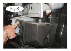
5. Remove the large black air box on the driver's side (two 10mm head bolts - Fig.K). Note: on some late model cars, you may not be able to remove the air box. If this is the case, remove the bolts and move the air box off to the side (Fig.L) to allow sufficient working room.
