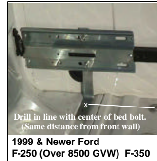
Drill in approximately center of slot, mid way between spot welds in bed floor.
